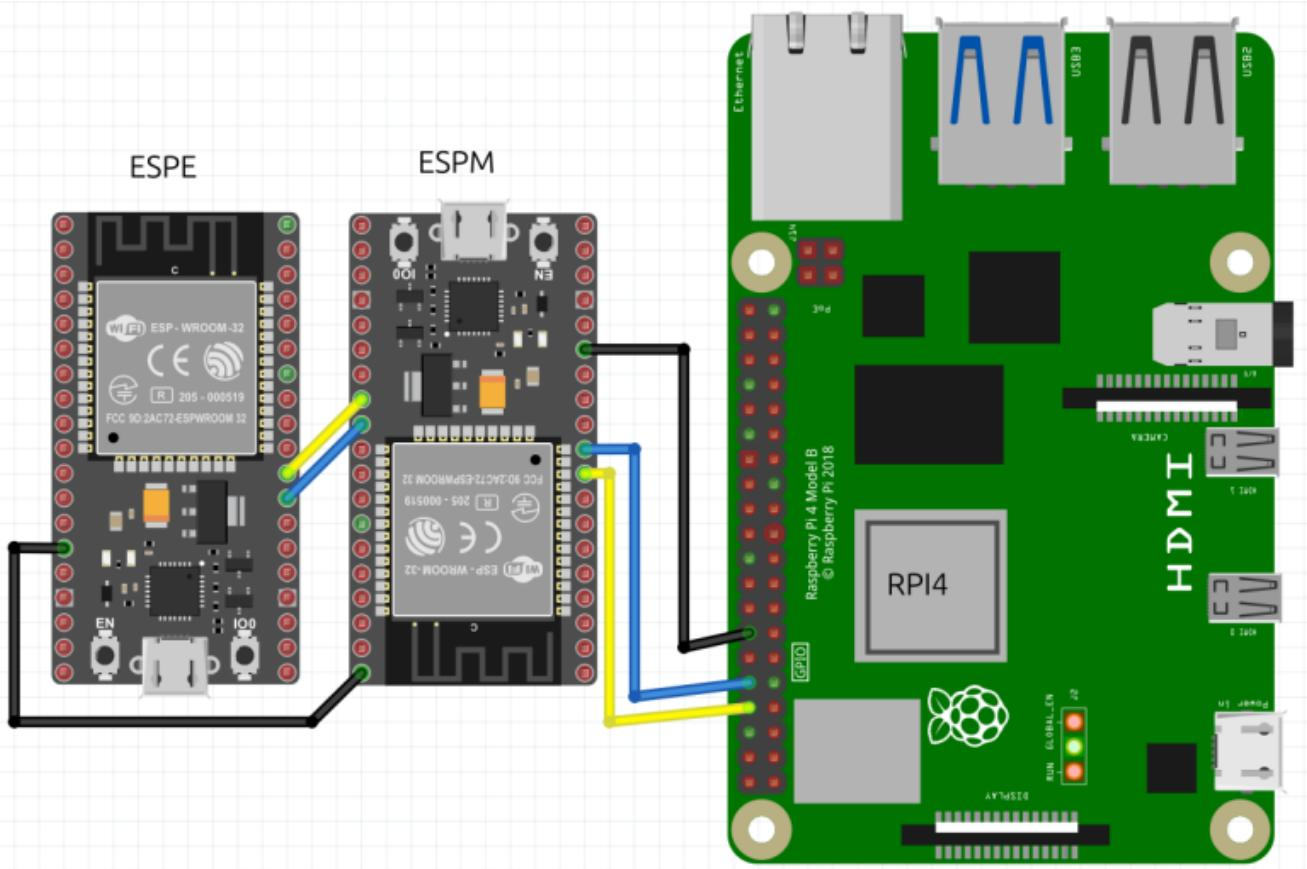
Raspberry Pi 4 → ESP32M ← ESP32E:
